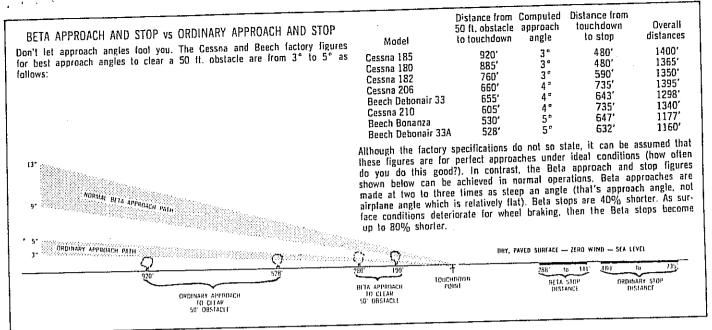
lines that can present a hazard in a long, flat approach. The attitude of the aircraft will be slightly nose down and rate of descent will vary from 500 to 1000 ft/min depending upon amount of Beta control being used. If control is moved past flat pitch position into reverse pitch, nose down attitude will increase somewhat and rate of descent can reach 2500 ft/min.
