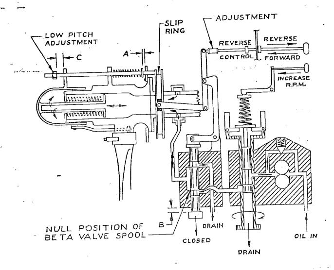
REVERSIBLE PROPELLER CONTROL SYSTEM DIAGRAM MODEL HC-92ZF-3
